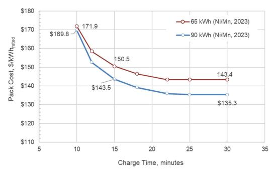
Figure 15. Pack cost (\$/kWh<sub>rated,2023</sub>) as a function of charging time, for a 65 kWh and 90 kWh NMC622-Graphite pack for MY2023.
